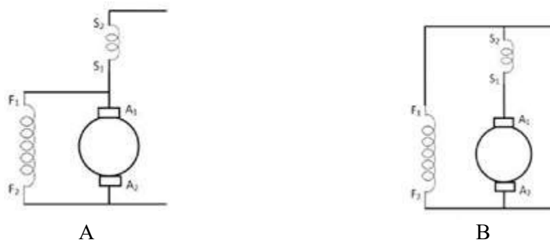
Fig. 1.19 A Schematic diagram of short -shunt compound machine
