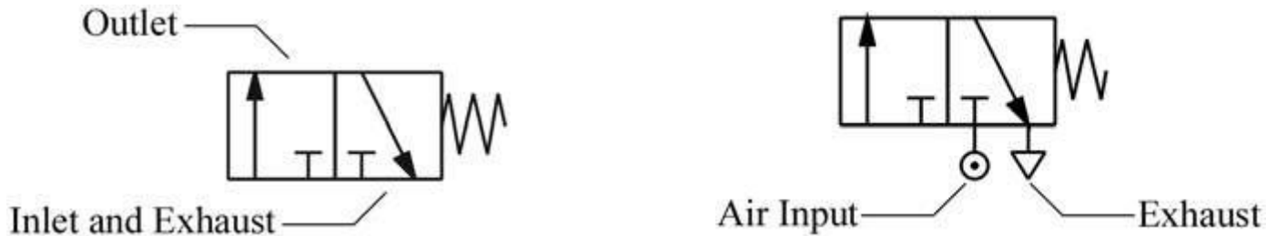
Fig 17 3/2 directional control valve (normally closed type)
