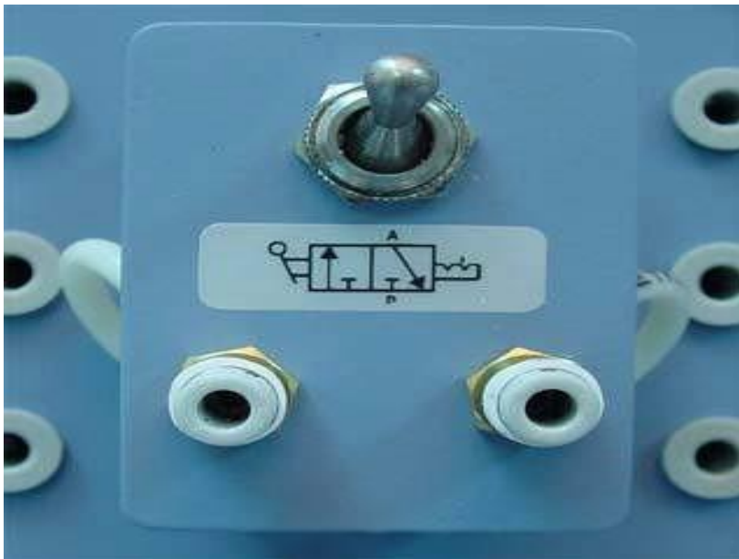
Fig. 10 (a) 3/2 directional control valve (b) Cross section
